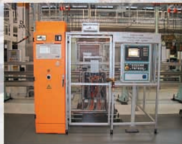
Timing cover assembly station and GardoTrans transport system fully integrated with m-Pro-400™.
